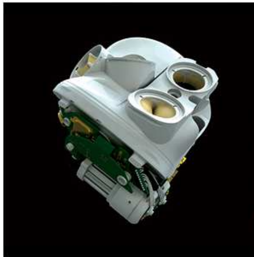
Cardio cyborg: This rendering shows the biological valves at the top of Carmat's artificial
